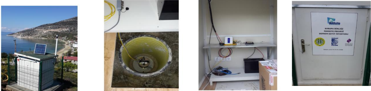
Figure 12: Instrumentation in the surface array stations (30 sec seismometer, solar panel, modem and battery etc.)
