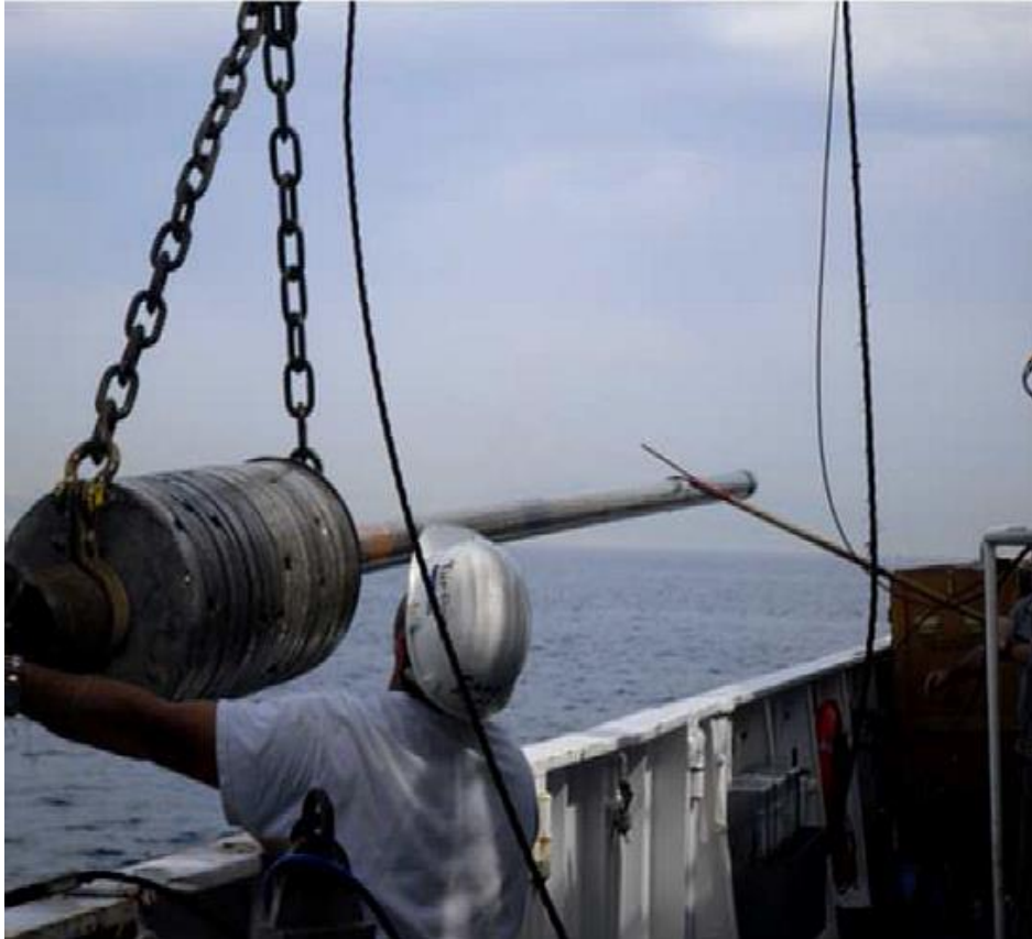
Figure 4. The 1.2 t gravity corer armed before a coring.
