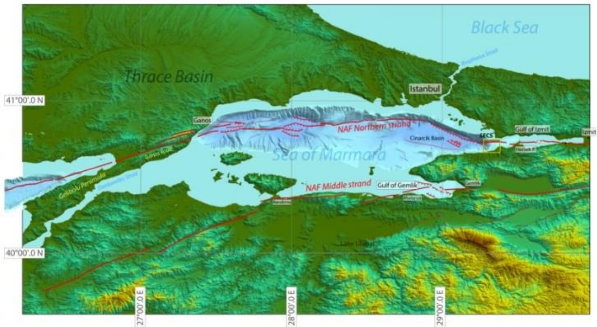
Figure 1. Structural map of the North Anatolian Fault (NAF) system in the Sea of Marmara. We note how the deep basins in Marmara form along the NAF northern strand. The study area is located at the western end of the Gulf of Izmit (yellow box). Modified from Gasperini et al., 2011.
