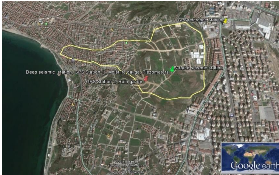
Figure 2: Positions of the different sensors of the observational monitoring system (yellow line is the landslide contour).
