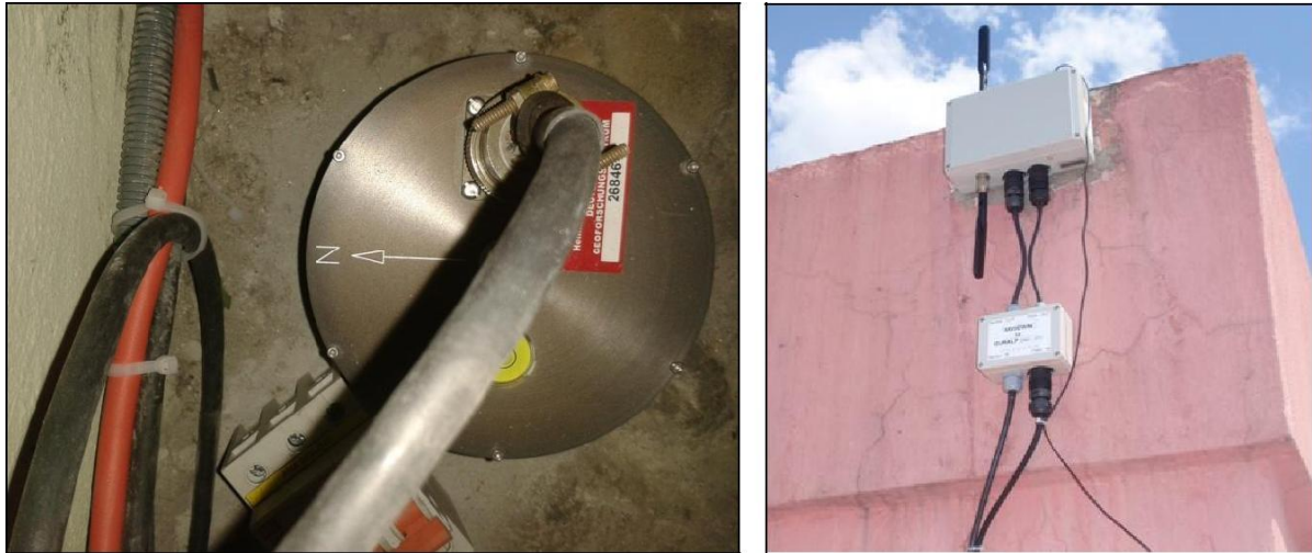
Figure 9: Location of the top floor Guralp sensor and SOSEWIN transducer in the B22 building
