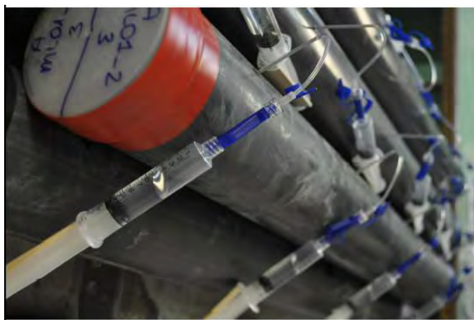
Figure II.22 : Pore fluid sampling using the rhyzon moisture sampler.
