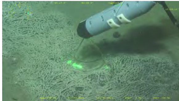
Figure II.6 : Chemical analysis of gas bubbles using a Raman spectrometer.
