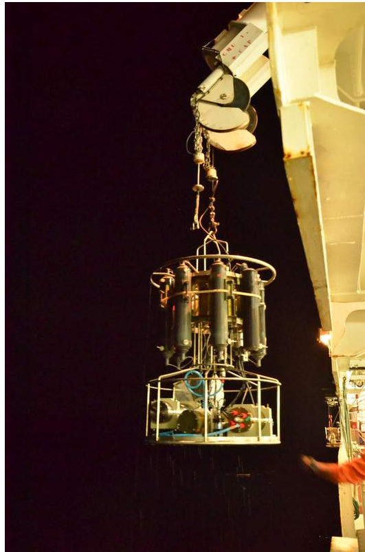
Figure II.20 : CTD- Hydrocast system equipped with methane sensors
