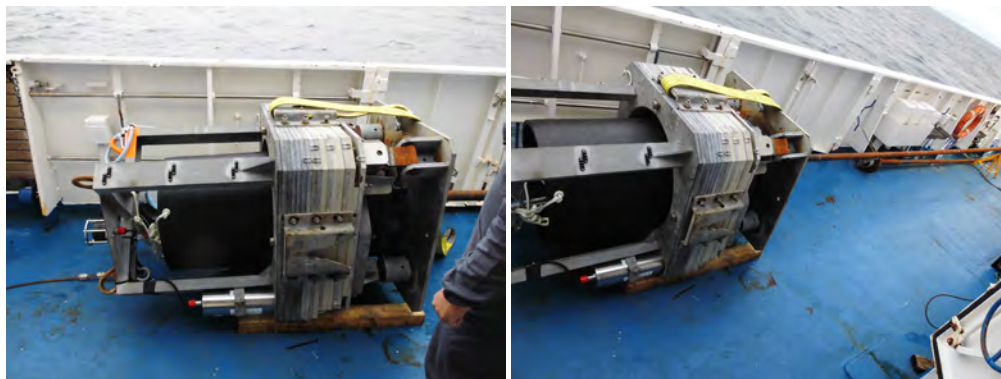
Figure 8: Head of Ifremer piezometer prior to deployment
