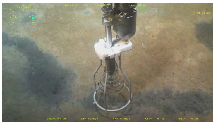
Figure II.4 : Gas sampling by ROV using a blade core.
